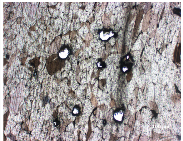
Chinese Copy Snorkel Material - distinctly grainy or crystal like structure where additive and colouring agents simply coat the base material. Consistency varies markedly throughout the part.
